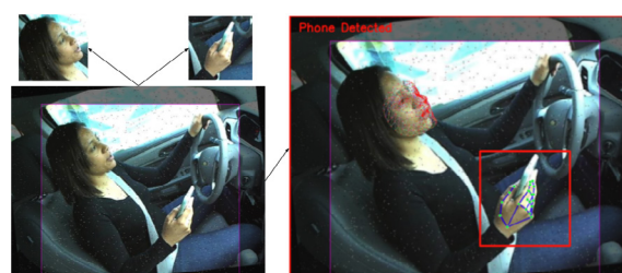
Figure 1: The bottom left picture displays a camera frame. The top left pictures show the cropped face and hand/phone captures. The right picture shows processed facial landmarks, hand landmarks, and a phone bounding box.
