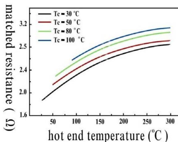
Figure 4: Matched Resistance Versus Hot End Temperature
