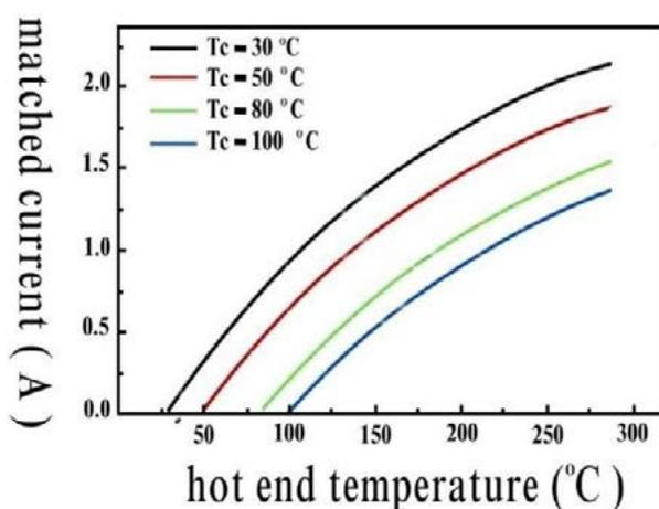
Figure 5: Matched Current Versus Hot End Temperature
