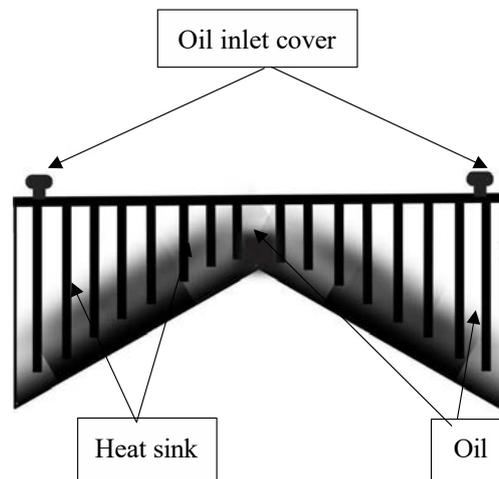
Figure 14: Heating Oil Tank of the Thermoelectric Generator
