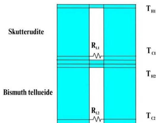
Figure 1: Model of The Two Stage Thermoelectric Generator
