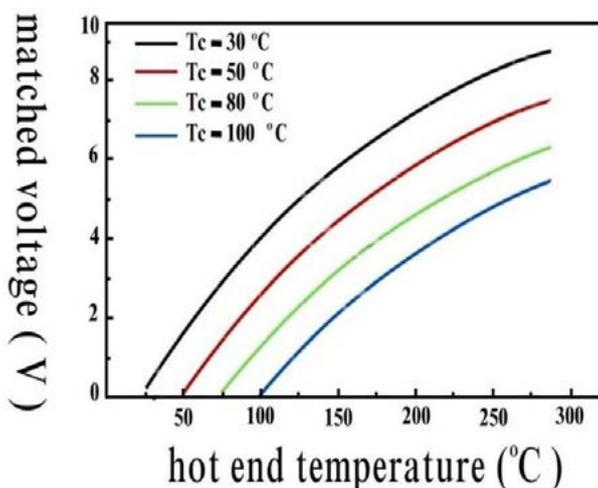
**Figure 3: Matched Voltage Versus Hot End Temperature**
