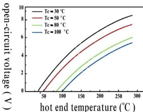
**Figure 2: Thevenin Voltage (Open-Circuit) Versus Hot end Temperature**
