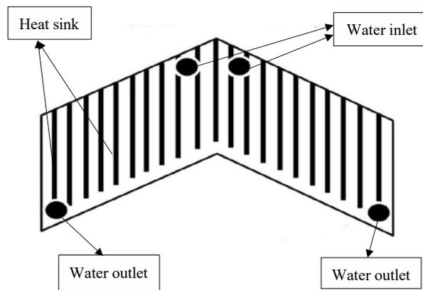
Figure 13: Cooling Tank of the Thermoelectric Generator
