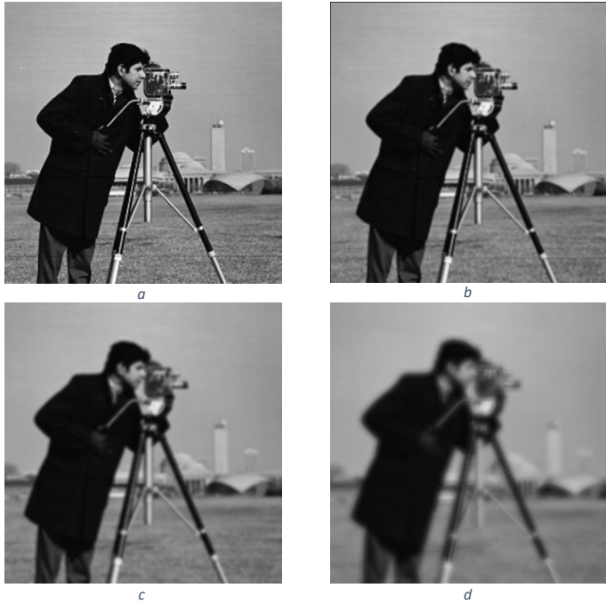
Figure 5: Comparing Original Image (a) and Applying 5*5 Filter (b), 10*10 Filter (c), and 15*15 Filter (d). As Expected, the Picture Gets More Smoothed as Size of Filter Increases.
