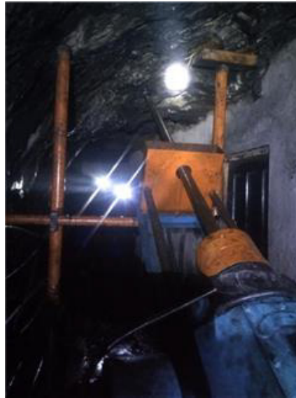
Figure 10: On-Site Mine Drilling with a Full-Hydraulic Mine Drilling Rig
