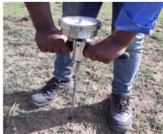
Figure 5: measuring soil resistance by cone penetrometer
