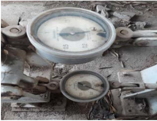
Figure 6: A dynamometer to measure the drawbar force
